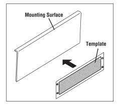
Cut and remove the hatching area on the template. Then drill four 1/8" mounting holes in the exact position according to the mounting paper.
